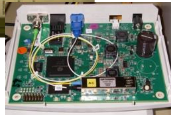
GPON ONT first prototype from Tellabs for 2.5/1.25Gbps using RSOA modules from France Telecom
