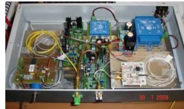
First prototype of the optical modules of 2.5 Gbps OLT based on DML
